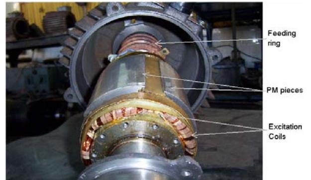
Fig. 8. HSM prototype rotor.
