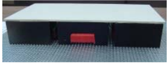
Figure 15 The laboratory model of the modular surface motor
