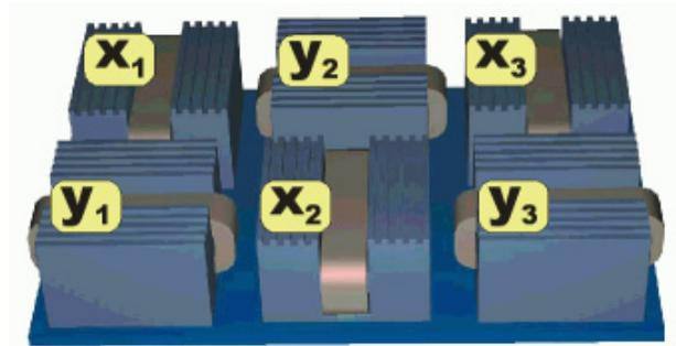
Fig. 4. The mover of the modular surface motor
