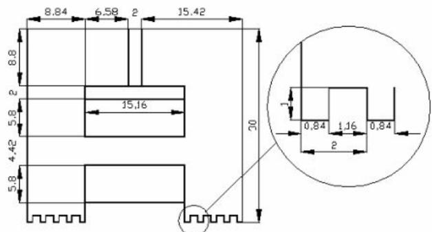
Fig. 12. The main dimensions of a module
