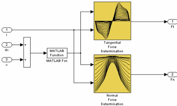
Fig. 9. The sub-system containing the model of one forcer module
