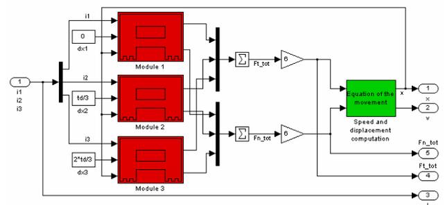
Fig. 8. The sub-system of the surface motor that ensures the movement on the x-axis
