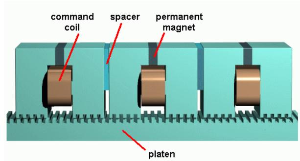
Fig. 3. The three-phase modular linear motor
