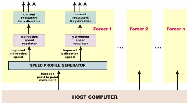
Fig. 6. The block diagram of the surface motor's control system
