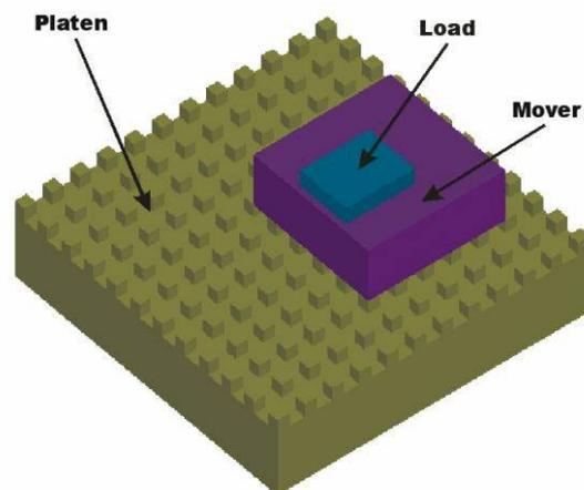
Fig. 5. The modular surface motor
