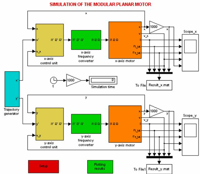
Fig. 7. The main window of the simulation program of the modular surface motor
