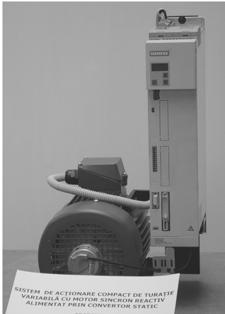
Fig. 5. The prototype of the intelligent compact drive system
