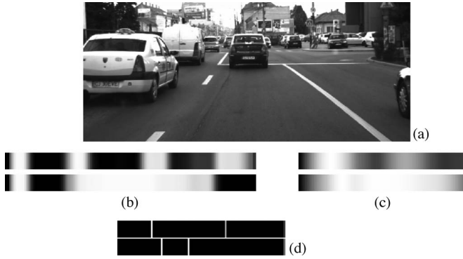
Fig. 7. Signal analysis. Left border is interrupted and right border is continuous. (a) Original grayscale image. (b) Filtered binary signal B . (c) Period histogram P . (d) First and second local maxima of P .
