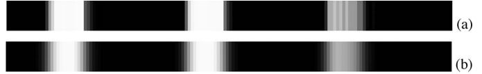
Fig. 6. (a) Time-integrated binary signal for the left boundary. (b) Result of Gaussian filtering of this signal.
