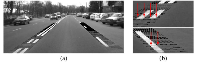
Fig. 9. Detection of double lines. (a) Search regions for counting marking/non-marking transitions. (b) Transitions on a search line.
