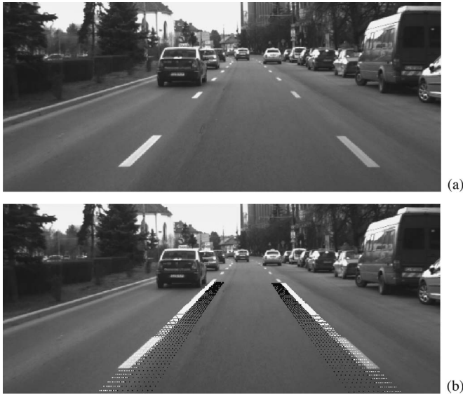
Fig. 4. (a) Original grayscale image. (b) Search areas for the markings (white dots) and for the asphalt reference grayscale values (black dots). The position of the search areas is given by a lane tracking result.
