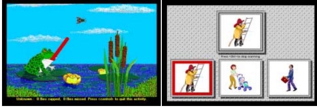
Figure 8: Sample games testing reaction time (left) and visual matching abilities (right). The red outlining box cycles through the options, and the user blinks when the matching image is outlined. Figure courtesy of Simtech Publications.
