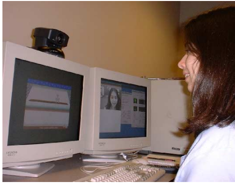
Figure 9: A user plays a scanning arcade game where the object is to throw a baseball at the plates on the shelf when they are outlined with a square. A long blink causes a ball to be thrown.
