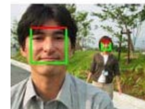
Figure 4: Example of detecting different sized faces.
