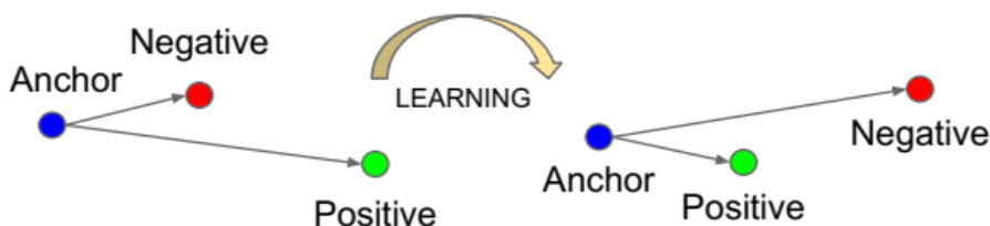
Figure 3. The Triplet Loss minimizes the distance between an anchor and a positive , both of which have the same identity, and maximizes the distance between the anchor and a negative of a different identity.
