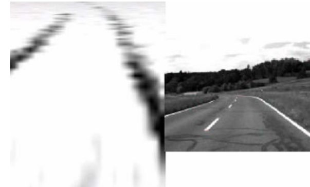
RADAR reflectivity 24GHz (SRR) / 77 (LRR)
