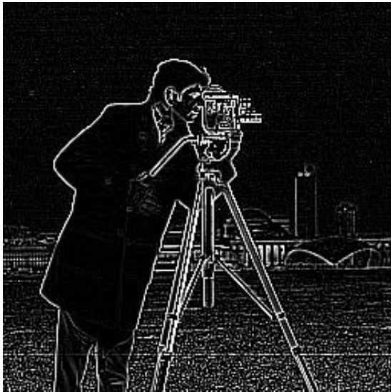
a. The result of applying the Laplace edge detection filter on the original image
