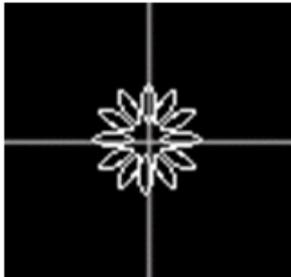
Figure 3. Gabor filter bank used in proposed method. The image represents the Fourier space. Ellipses denote the half-response for each filter. Note how the half-response regions of each filter touches with the adjacent ones.
