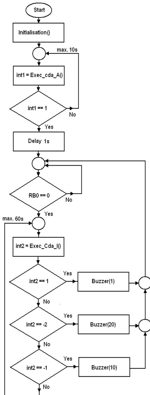
Figure 7. The logical diagram of the firmware
