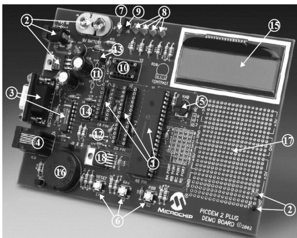
Figure 5. The demonstration board PICDEM 2 PLUS
