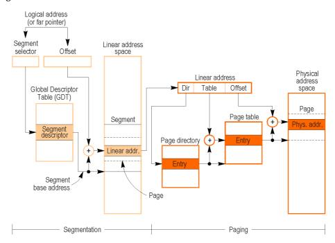
Figure 4.62. Segmentation and paging for the Intel Architecture
