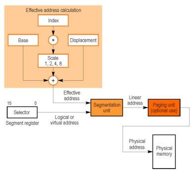
Figure 4.61. Address translation for the Intel Architecture
