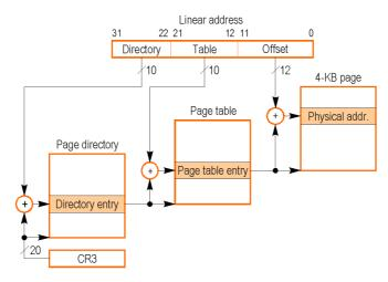
**Figure 4.63.** Linear address translation for the *Intel Architecture* (4-KB pages).
