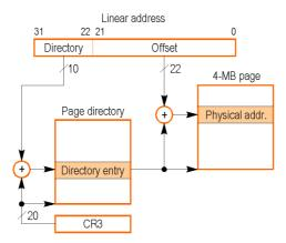
**Figure 4.64.** Linear address translation for the *Intel Architecture* (4-MB pages).
