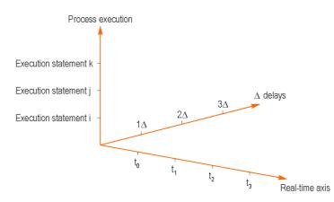
Figure 2.8. Three dimensions of time in VHDL.
