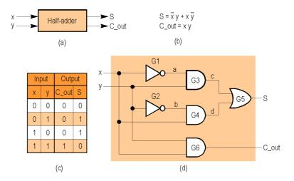
**Figure 2.4.** Different representations of a half adder: (*a*) block symbol; (*b*) Boolean equations; (*d*) truth table; (*d*) logic diagram.
