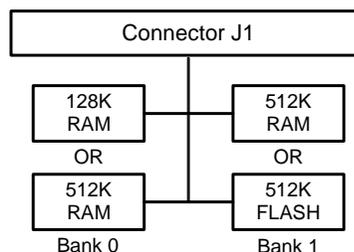
Mem1 circuit board block diagram
