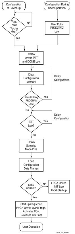
Figure 14: Configuration Flow Diagram
