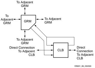
Figure 7: Spartan-IIE Local Routing
