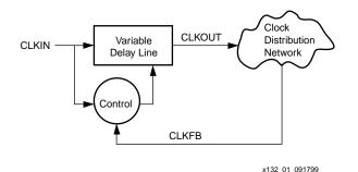
Figure 10: Delay-Locked Loop Block Diagram
