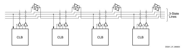
Figure 8: BUFT Connections to Dedicated Horizontal Bus Lines
