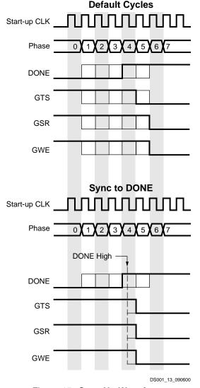
Figure 15: Start-Up Waveforms
