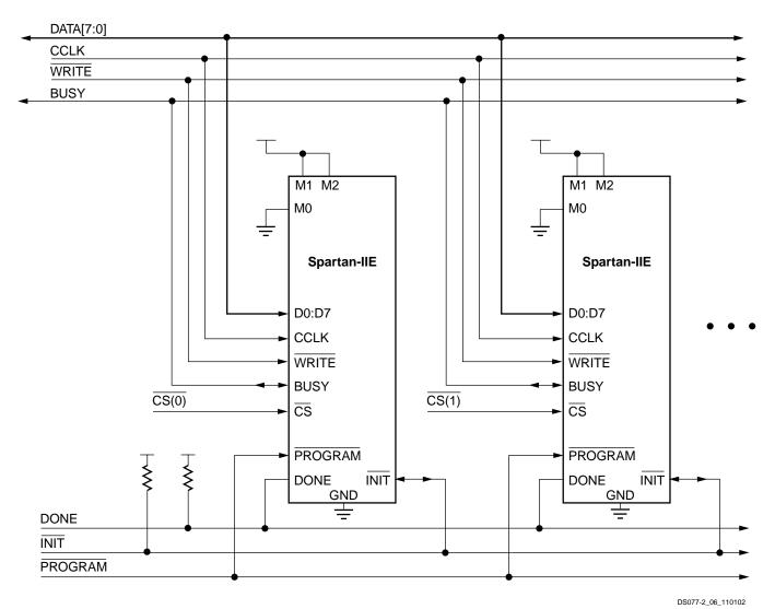
Figure 18: Slave Parallel Configuration Circuit Diagram
