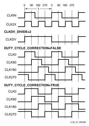
Figure 11: DLL Output Characteristics
