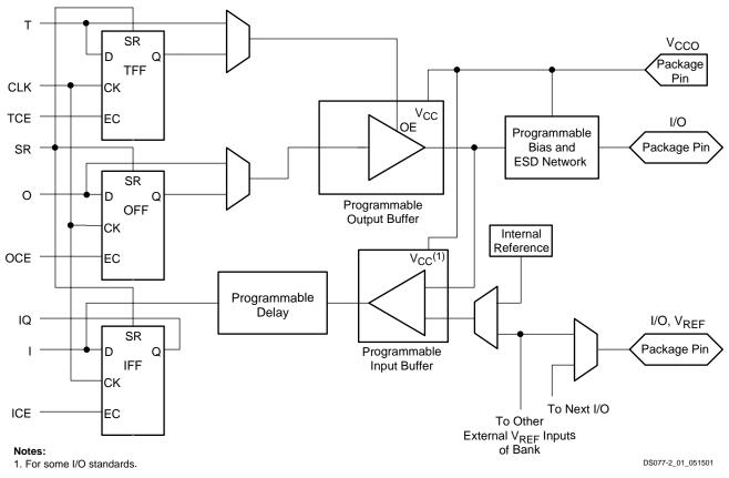
Figure 2: Spartan-IIE Input/Output Block (IOB)
