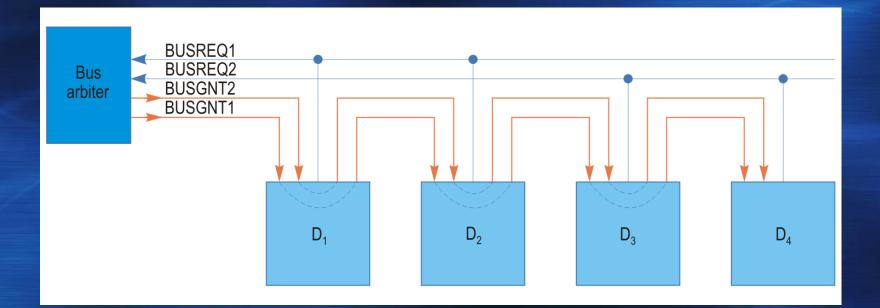
Each device attaches to one of the bus request lines, according to the device priority
