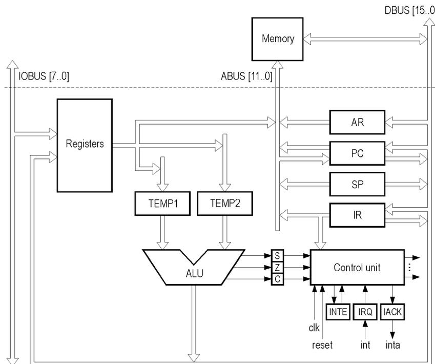
**Figure 2.** Block diagram of the ConP processor.
