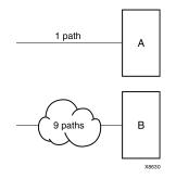
If an error is generated at the endpoints of A and B, the timing report would lists one error for each of the end points.
