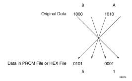
In a bitstream contained in a BIT file, the Least Significant Bit (LSB) is always on the left side of a byte. But when a PROM programmer or a microprocessor reads a data byte, it identifies the LSB on the right side of the byte. In order for the PROM programmer or microprocessor to read the bitstream correctly, the bits in each byte must first be swapped so they are read in the correct order.
