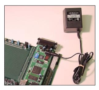
Or you can attach the 9V DC power supply directly to jack J7 on the XStend Board. Now the XSA Board will draw its power from the XStend Board.
