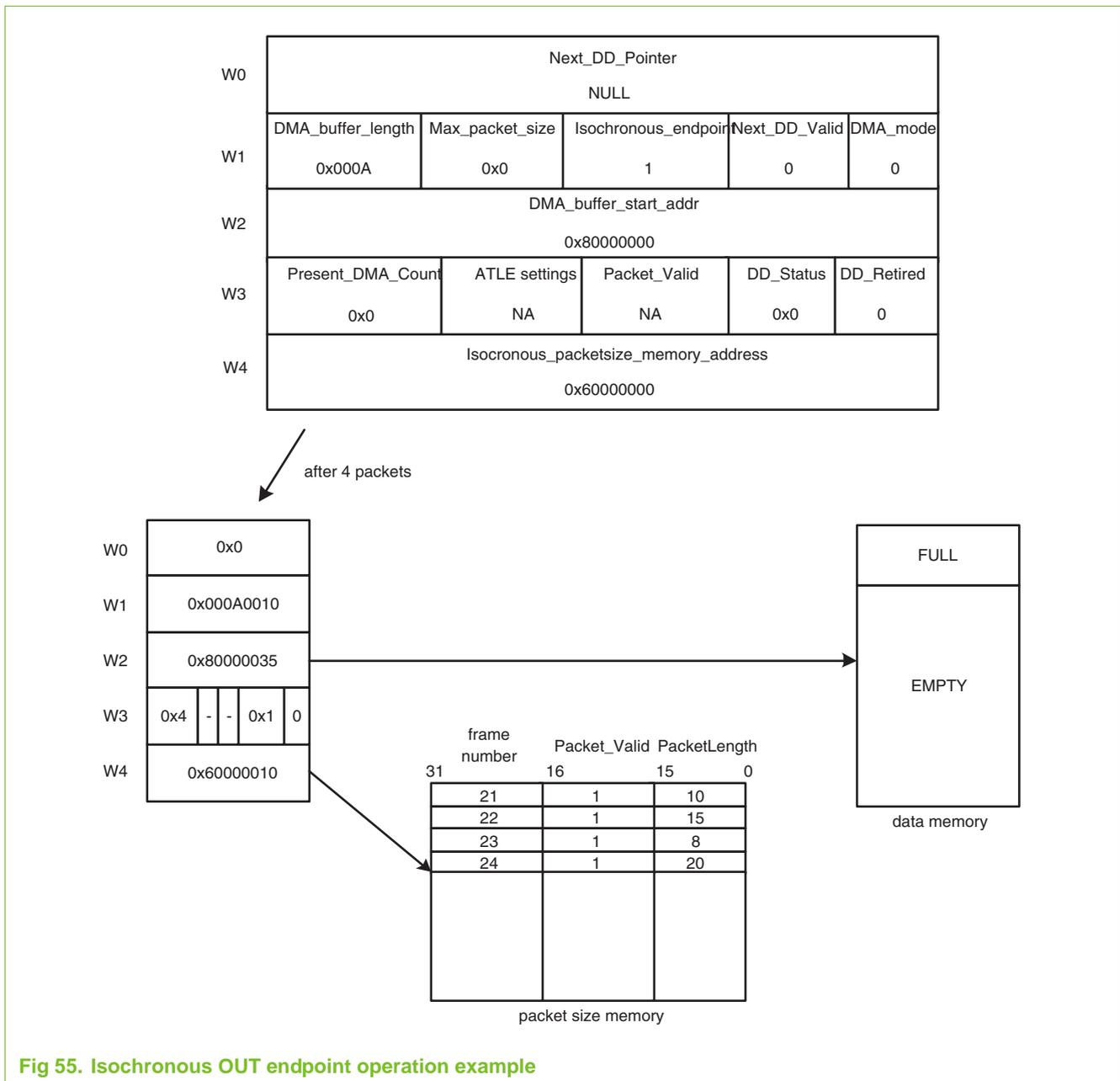
Fig 55. Isochronous OUT endpoint operation example
