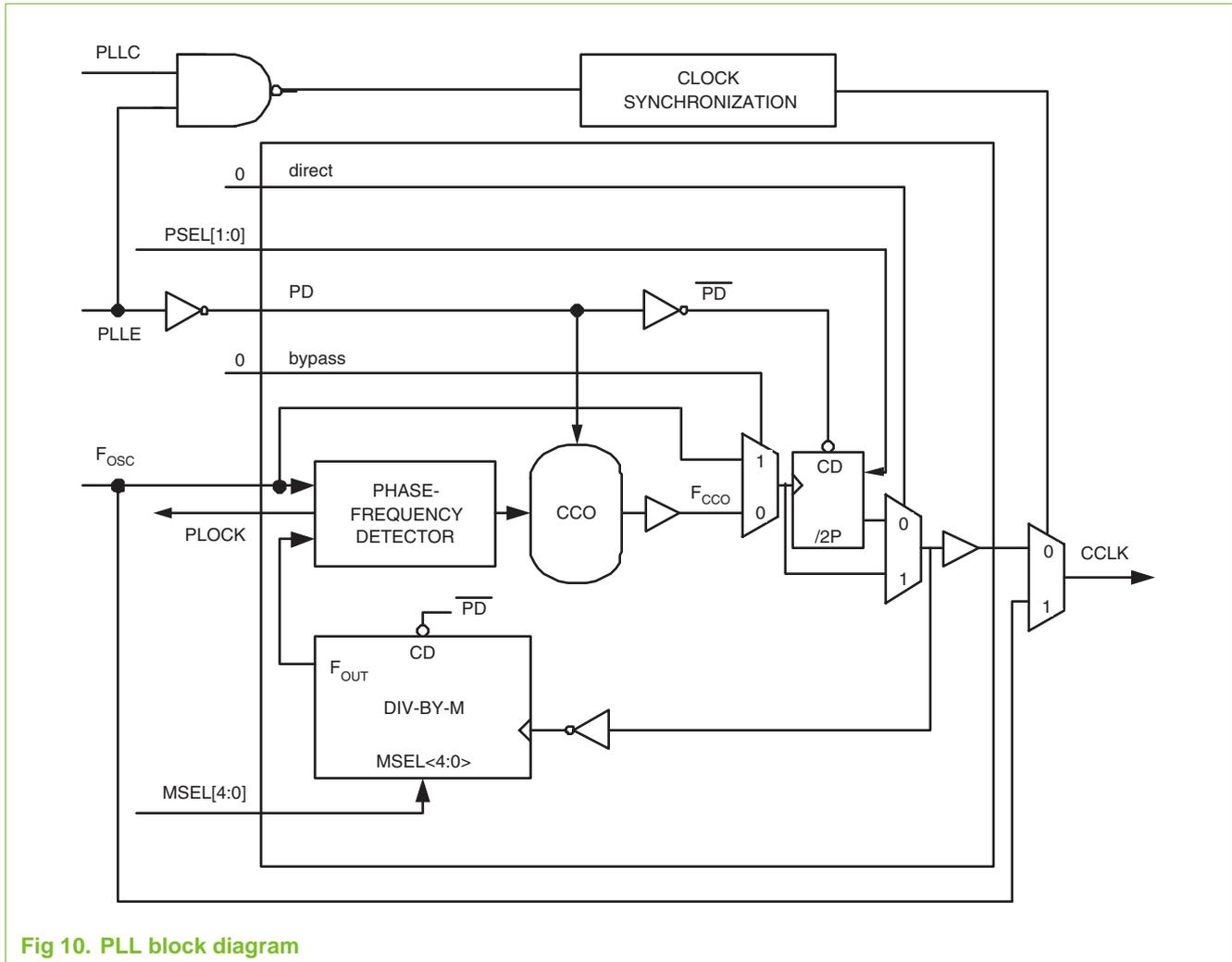
Fig 10. PLL block diagram
