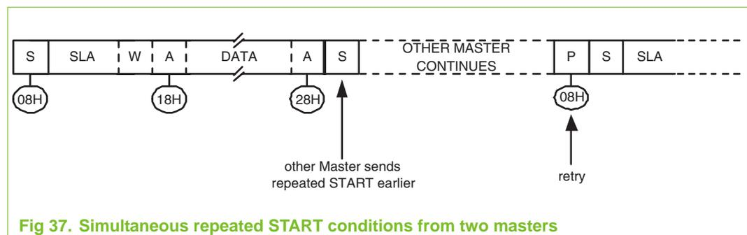
Fig 37. Simultaneous repeated START conditions from two masters
