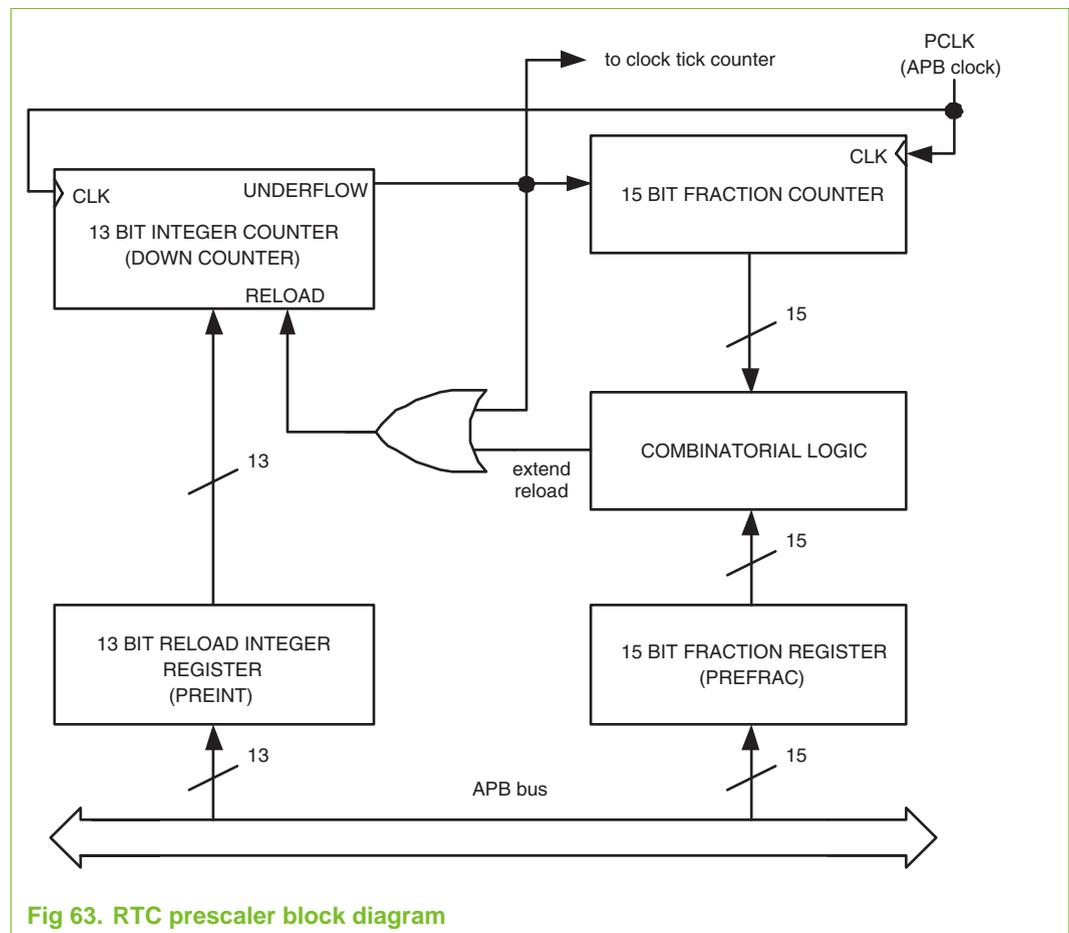
Fig 63. RTC prescaler block diagram
