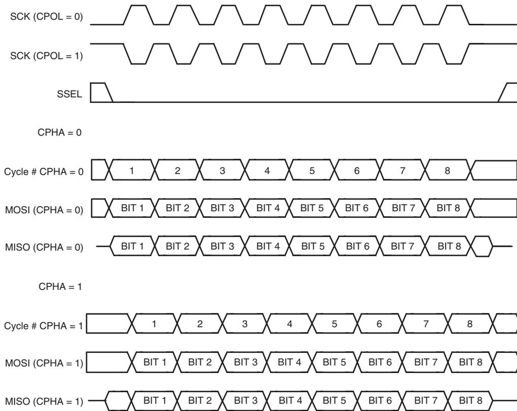
Fig 40. SPI data transfer format (CPHA = 0 and CPHA = 1)
