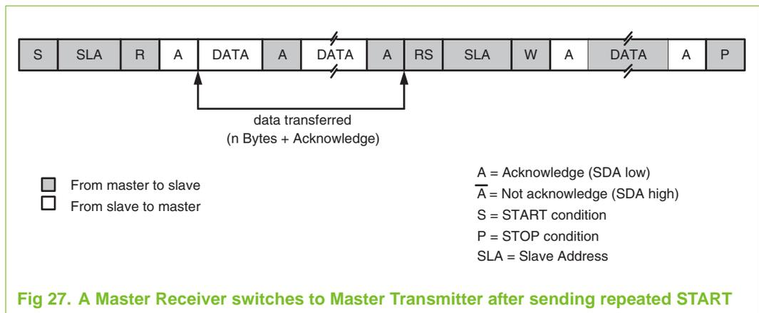
Fig 27. A Master Receiver switches to Master Transmitter after sending repeated START
