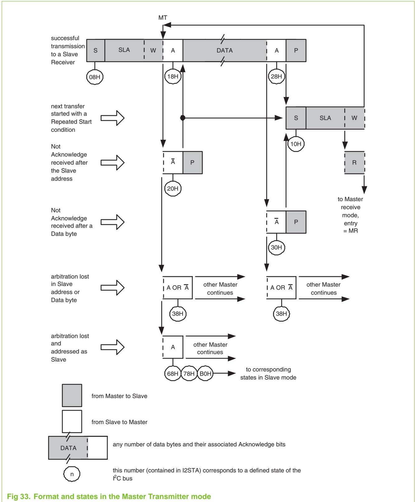
Fig 33. Format and states in the Master Transmitter mode
