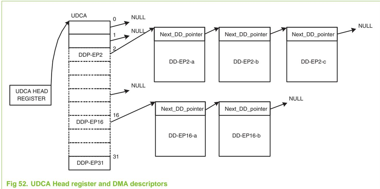
Fig 52. UDCA Head register and DMA descriptors
