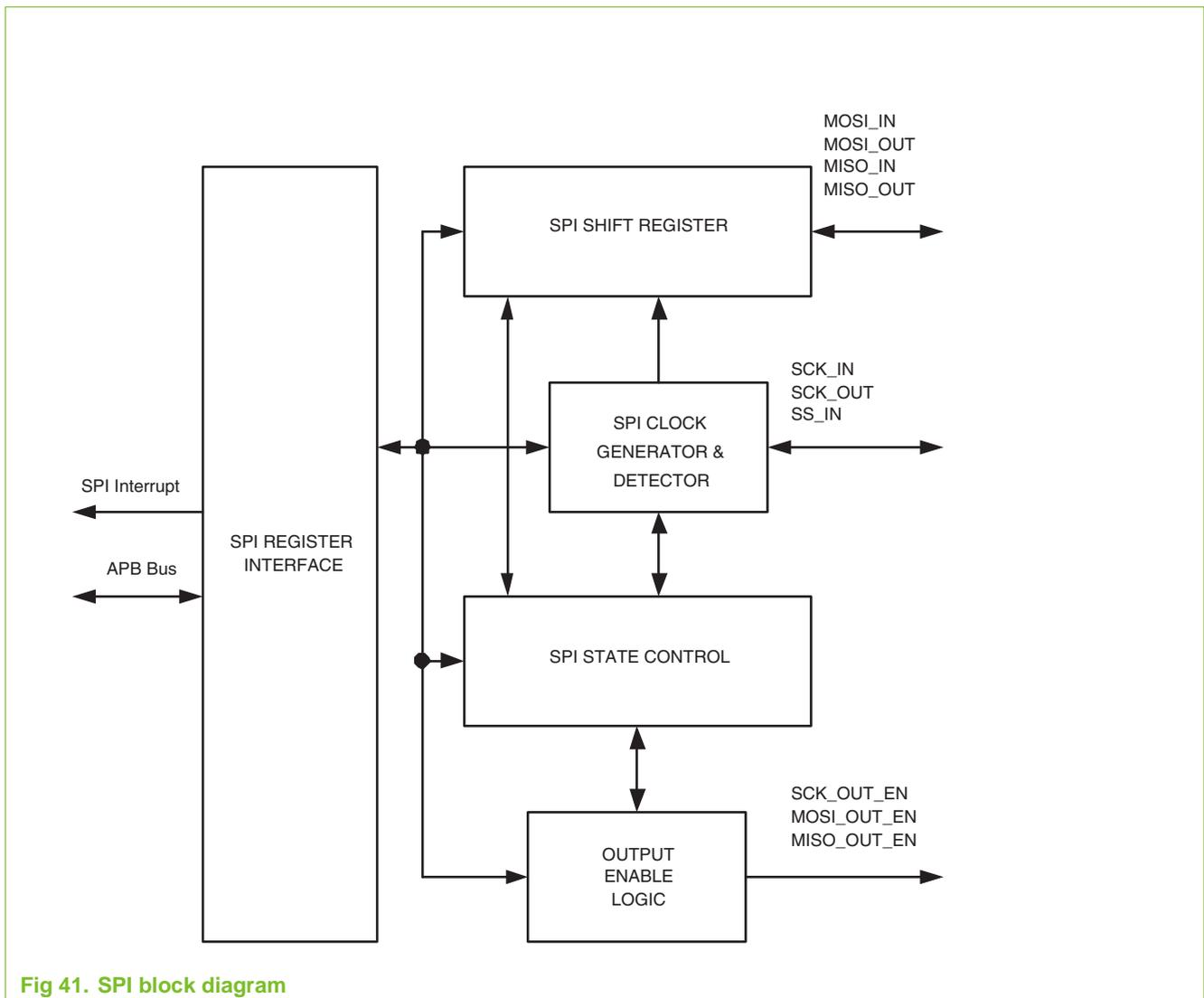
Fig 41. SPI block diagram
