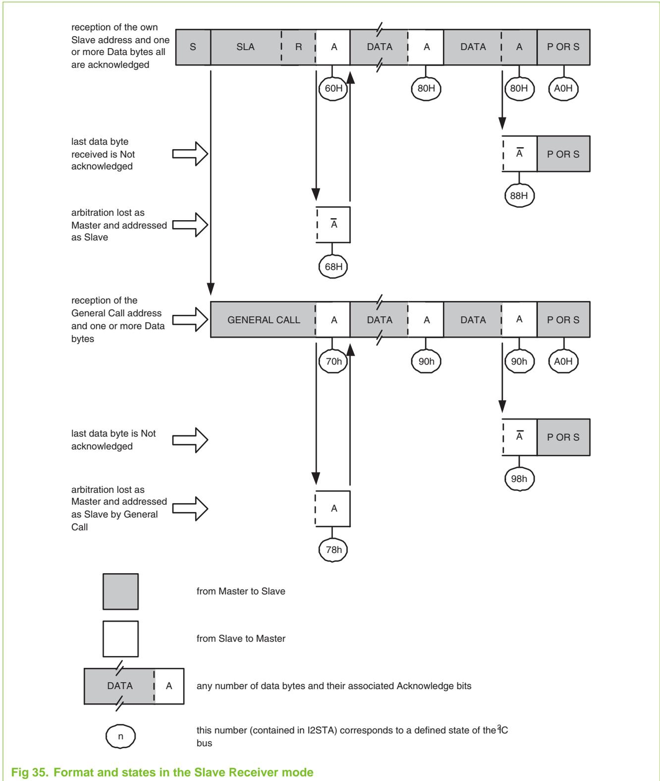
Fig 35. Format and states in the Slave Receiver mode
