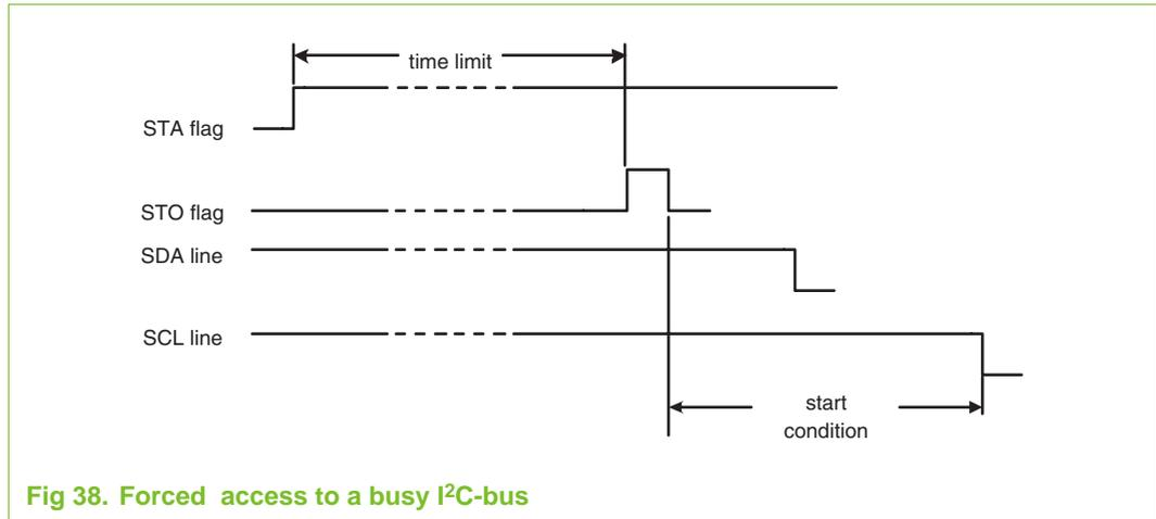
Fig 38. Forced access to a busy I<sup>2</sup>C-bus
