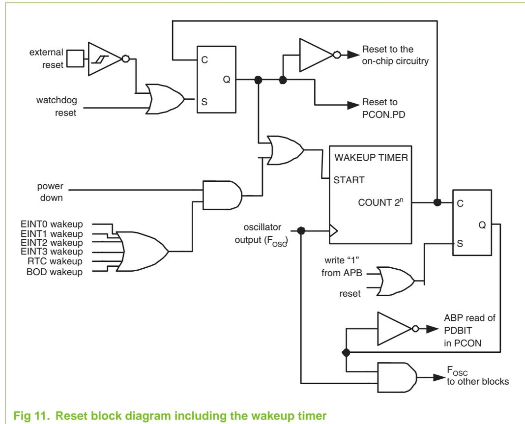
Fig 11. Reset block diagram including the wakeup timer
