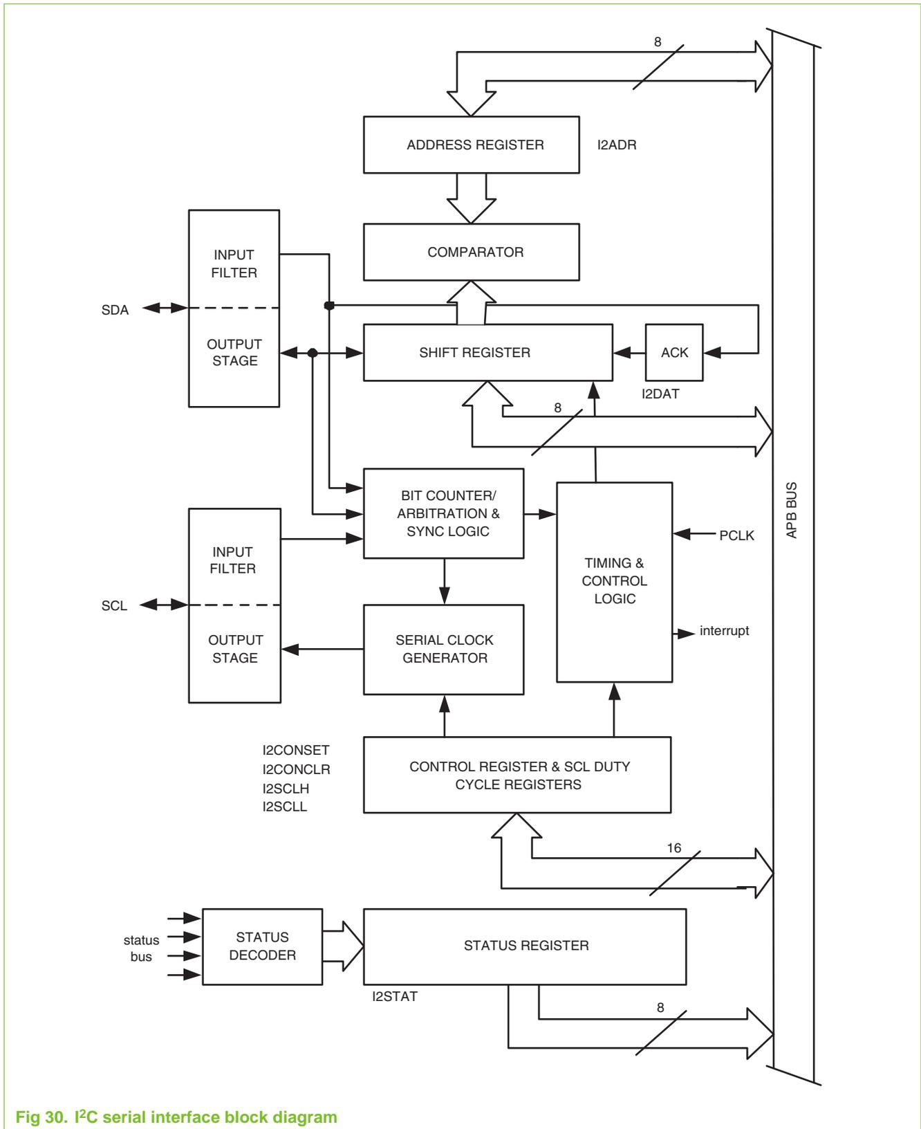
Fig 30. I<sup>2</sup>C serial interface block diagram
