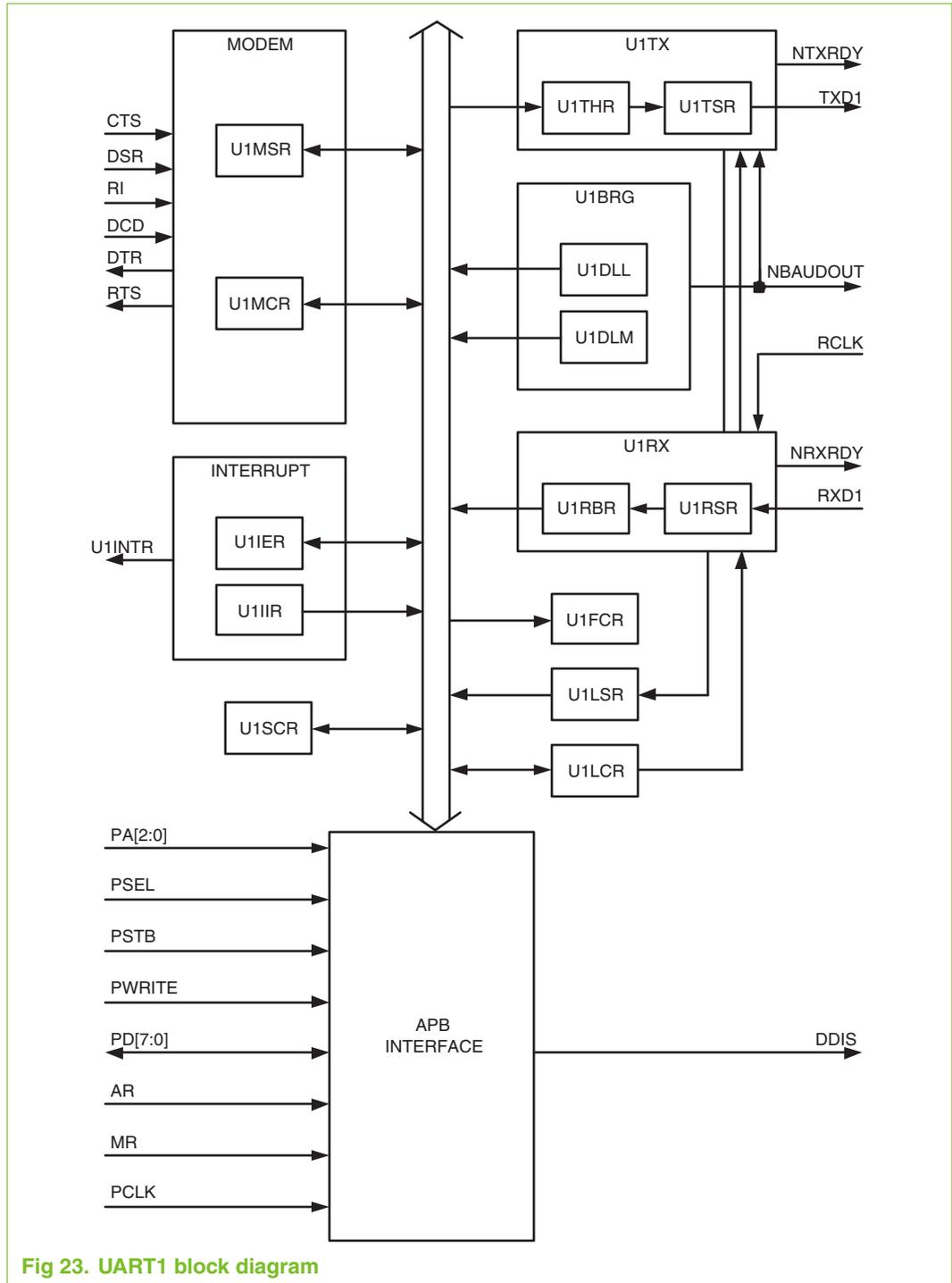
Fig 23. UART1 block diagram
