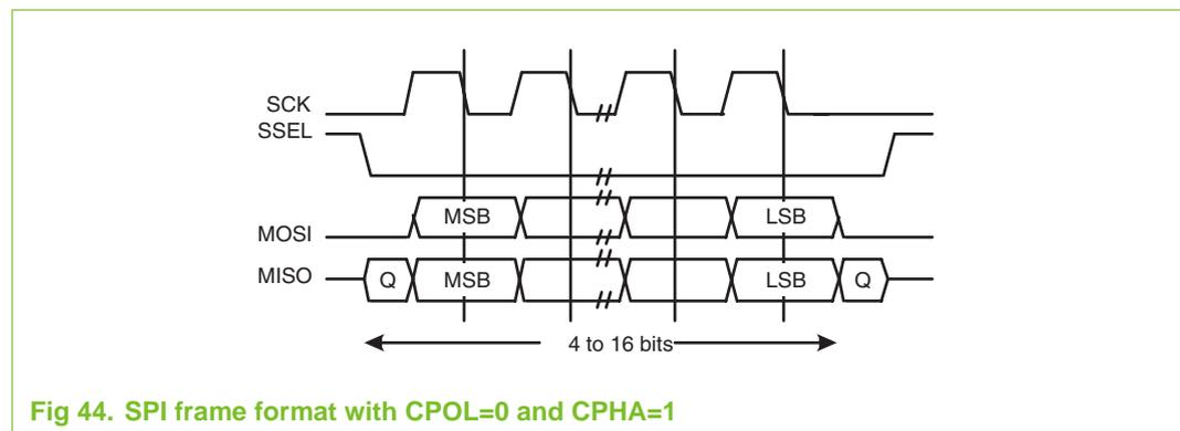
Fig 44. SPI frame format with CPOL=0 and CPHA=1
