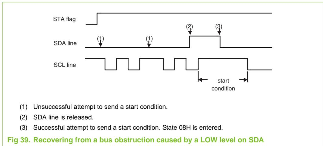
Fig 39. Recovering from a bus obstruction caused by a LOW level on SDA
