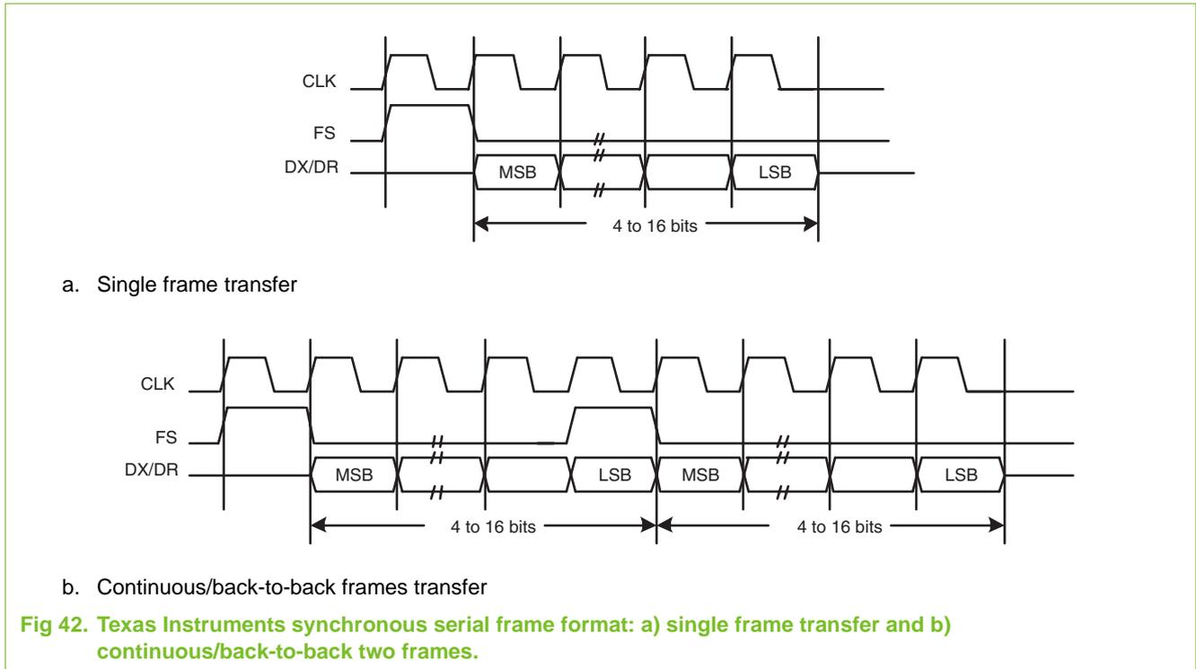
**Fig 42. Texas Instruments synchronous serial frame format: a) single frame transfer and b) continuous/back-to-back two frames.**
