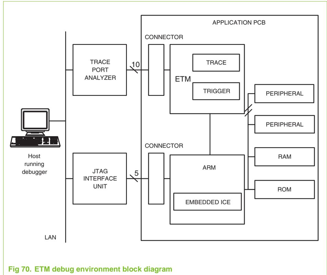
Fig 70. ETM debug environment block diagram
