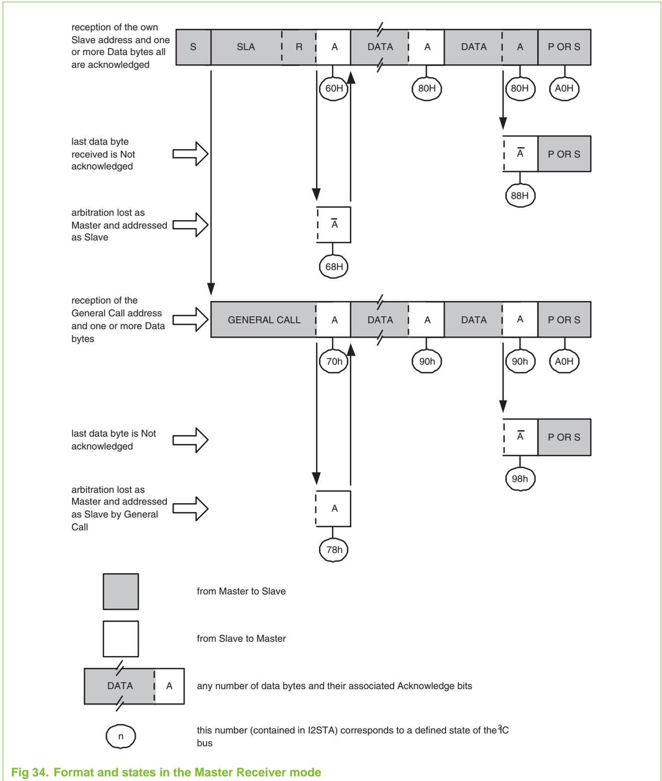
Fig 34. Format and states in the Master Receiver mode
