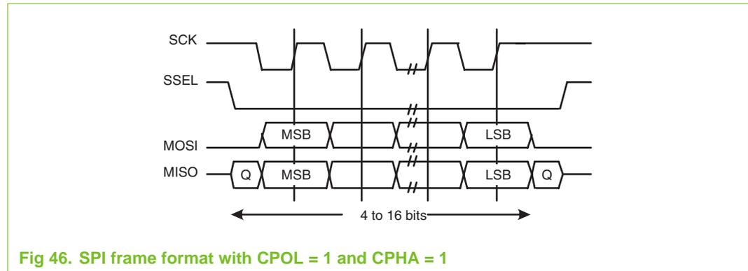
Fig 46. SPI frame format with CPOL = 1 and CPHA = 1
