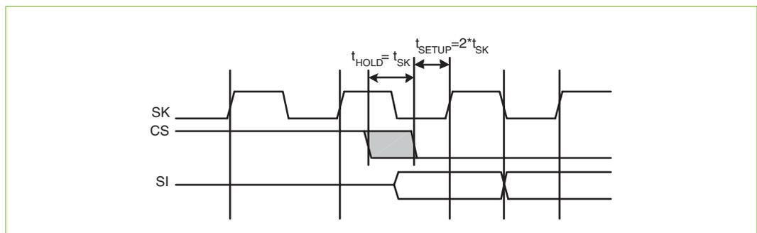
Fig 49. Microwire frame format (continuous transfers, details)
