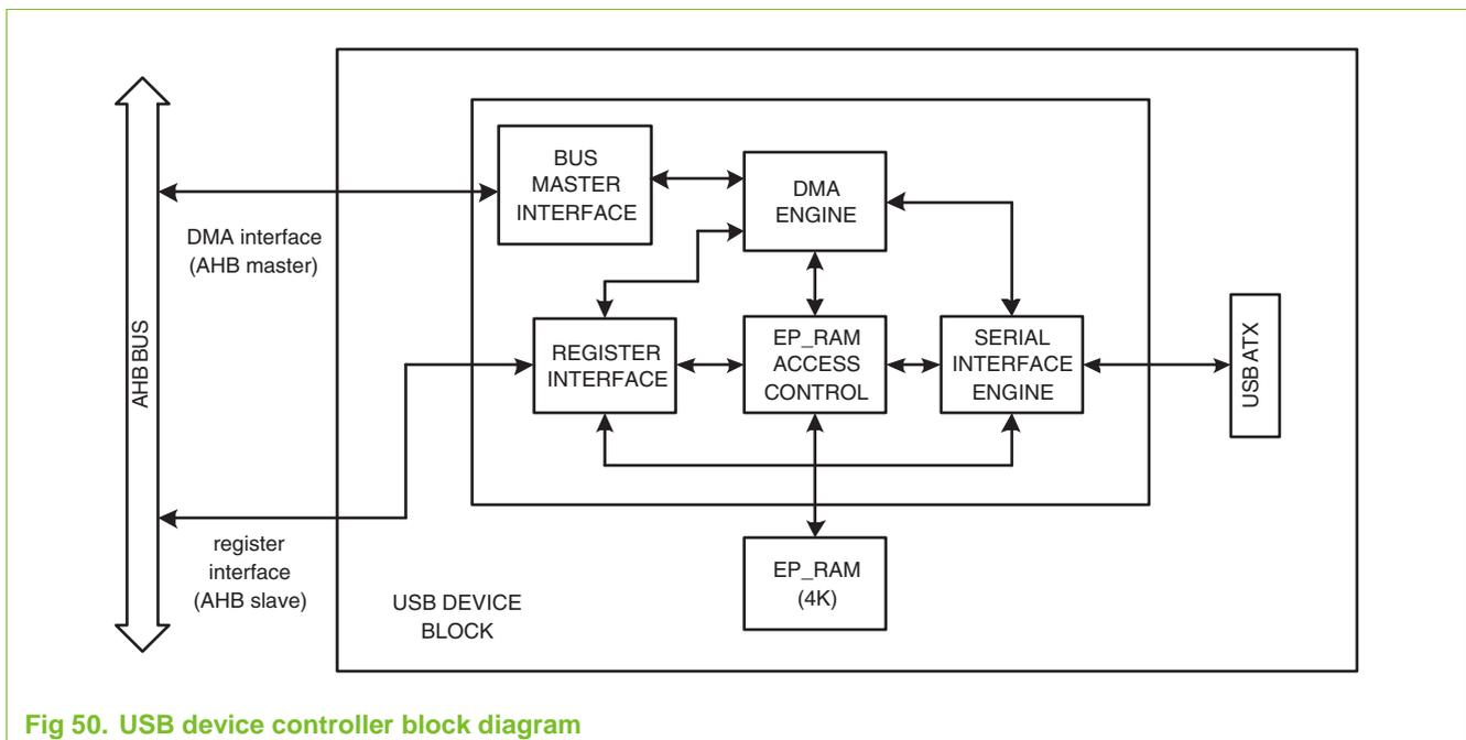
Fig 50. USB device controller block diagram
