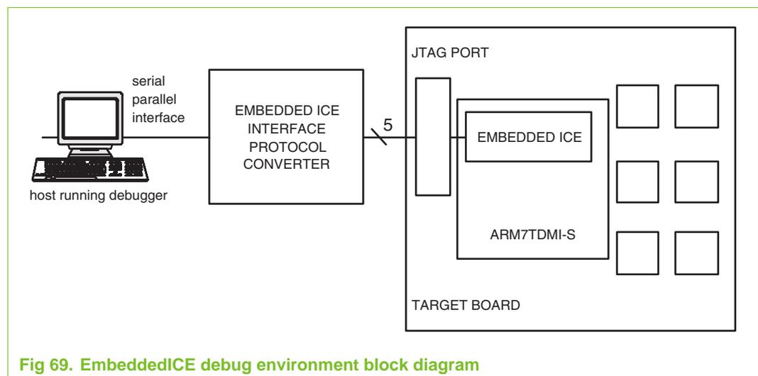
**Fig 69. EmbeddedICE debug environment block diagram**
