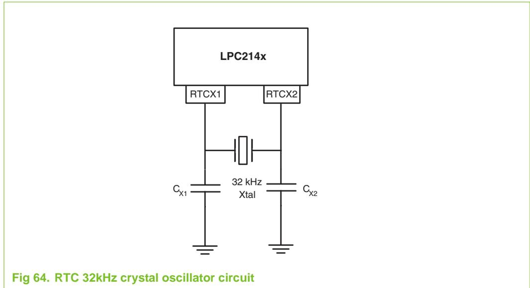
Fig 64. RTC 32kHz crystal oscillator circuit
