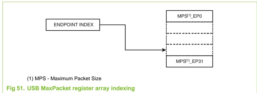
**Fig 51. USB MaxPacket register array indexing**
