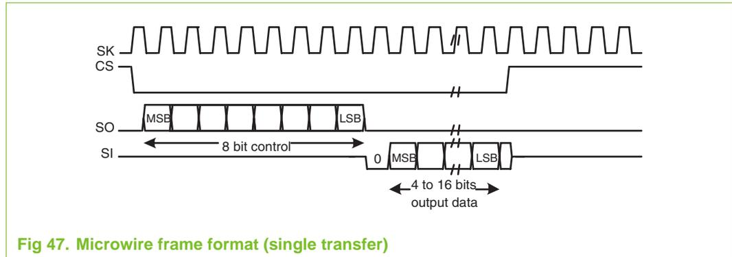
Fig 47. Microwire frame format (single transfer)
