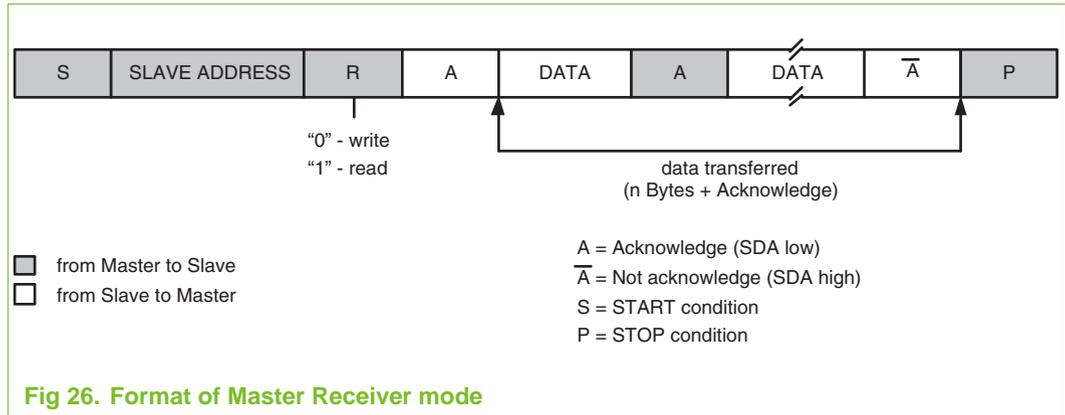
Fig 26. Format of Master Receiver mode
