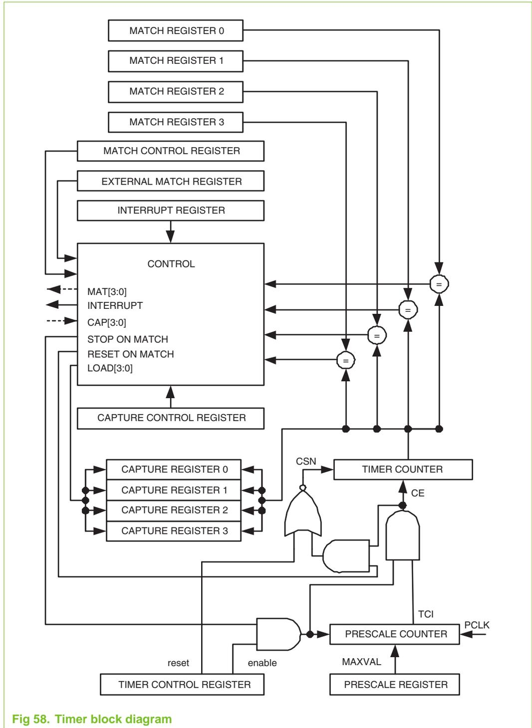
Fig 58. Timer block diagram
