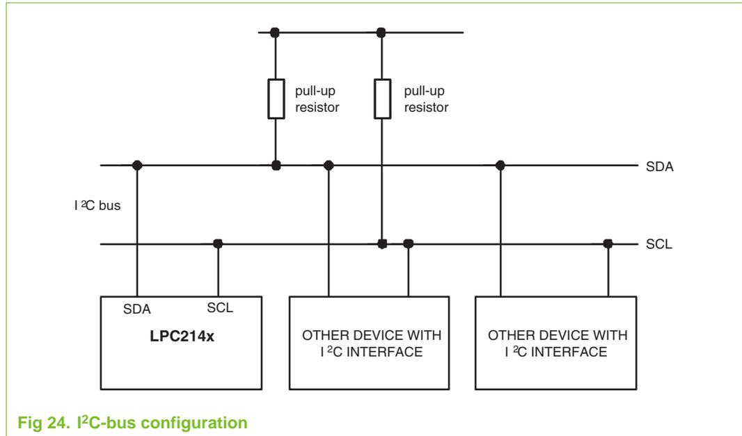
Fig 24. I<sup>2</sup>C-bus configuration
