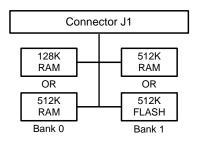
Mem1 circuit board block diagram
