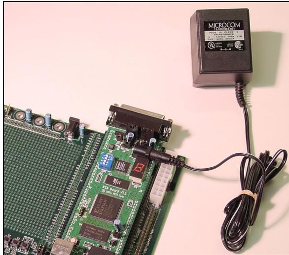
Or you can attach the 9V DC power supply directly to jack J7 on the XStend Board. Now the XSA Board will draw its power from the XStend Board.
