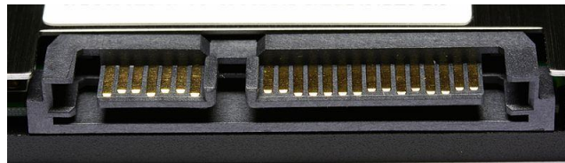
Figure 7.2. Standard combo SATA connector of a disk drive.
