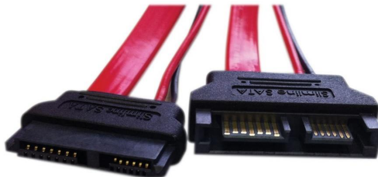
Figure 7.3. Mini-SATA combo connectors of a SATA cable.
