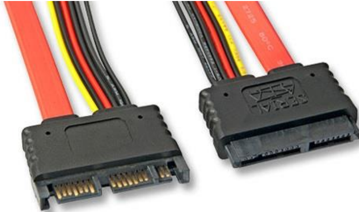
Figure 7.4. Micro-SATA combo connectors of a SATA cable.
