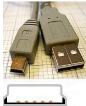
Figure 4.9. Mini-B USB plug near a Type-A plug.
