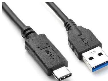
Figure 4.13. USB Type-C and Type-A plugs.
