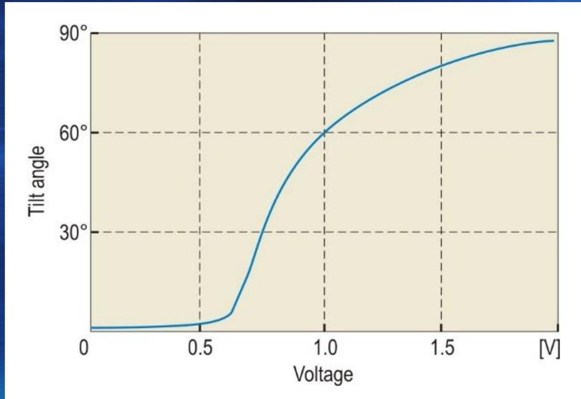
Response of a **TN** cell to an applied voltage
