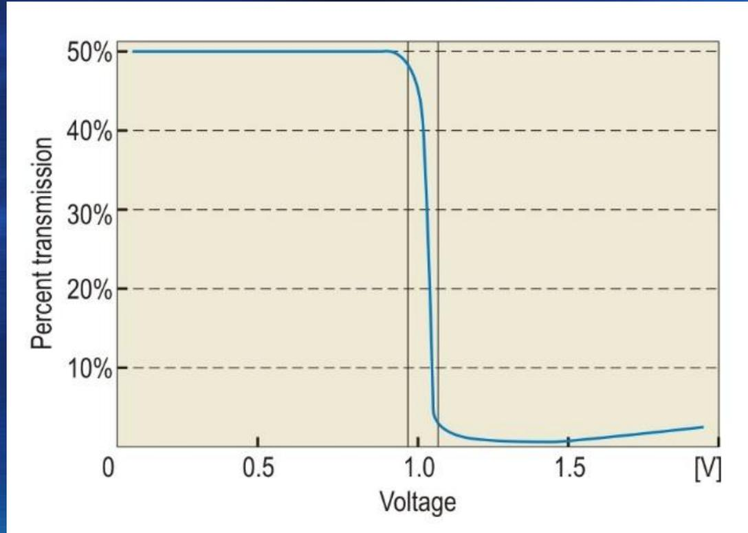
Percent transmission of light for an **STN** cell with a twist angle of  $270^\circ$
