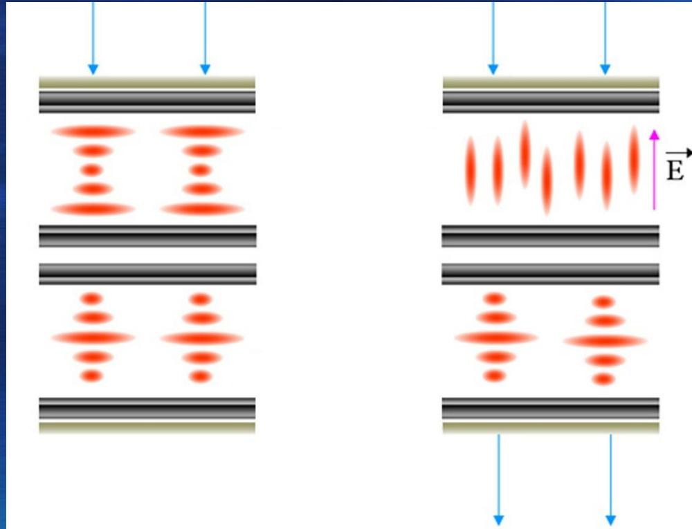
DSTN cell in OFF state (left) and ON state (right)
