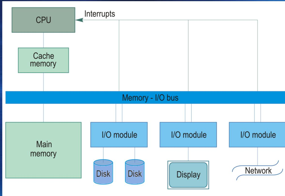
Structure of a computer system and a typical I/O system
