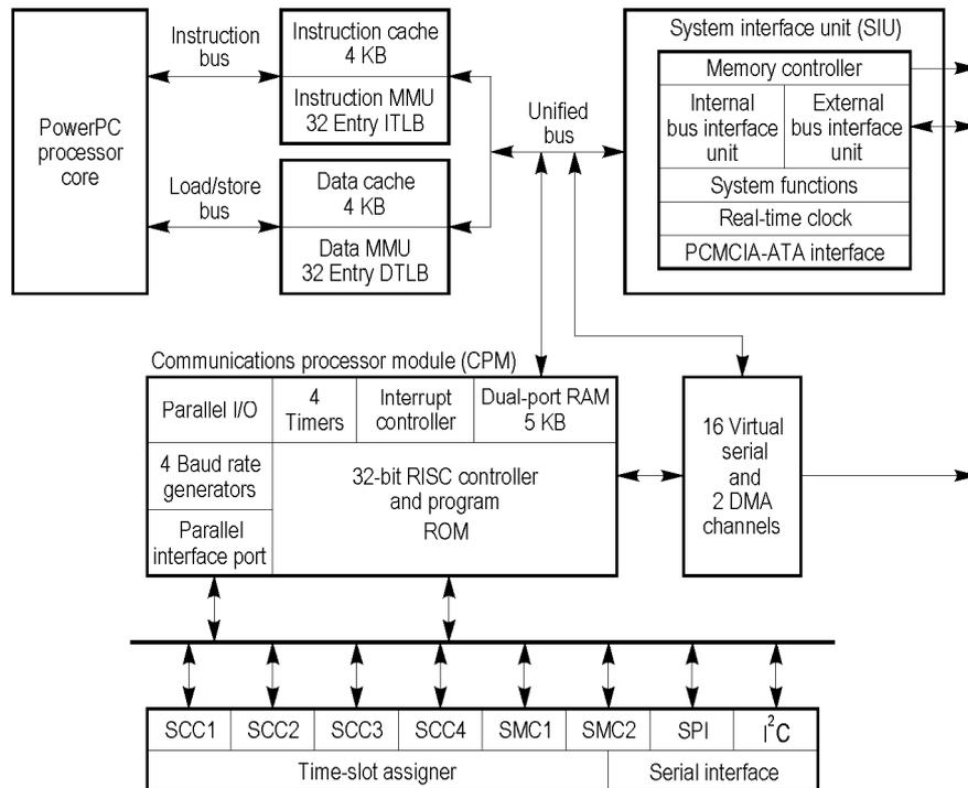
Figure 6.18. Block diagram of the MPC860 processor.
