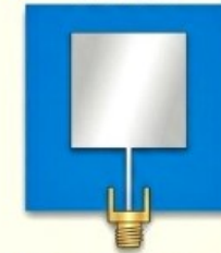
(e) Rectangular patch Use: General purpose, low-cost applications
