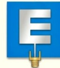
(h) E-shaped patch Use: Dual-band and multi-band mobile communications
