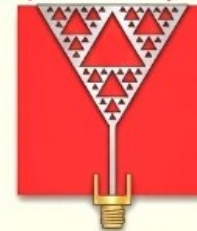
(g) Fractal Use: Miniaturization and multi-band operation
