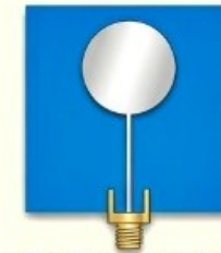
(b) Circular patch Use: Circular polarization and radar
