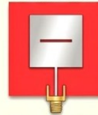
(d) Slot insertion Use: Multi-band and dual-polarization operation
