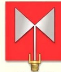
(a) Bow-tie Use: UWB and wideband communications
