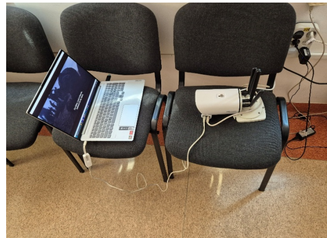
Figure 7. Testbed setup for Dynamic PRB allocation with CCTV camera and B200 USRP@ 1m
