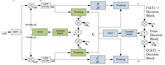
Figure 9. DDbased recovery and synchronization of the local carrier and symbol clock
