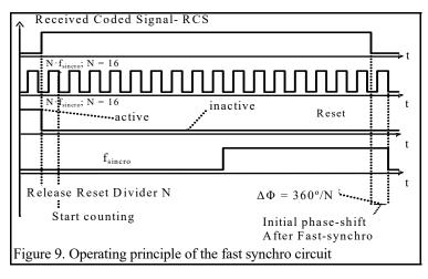
This fact makes the negative transition of the  $f_{synchro}$  to occur with a delay of maximum  $\Delta\Phi_{max}$ , compared to the arriving moment of the second transition of the RCS, see fig. 19 and (7):
