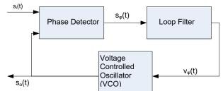
Figure 1. Block diagram of a PLL
