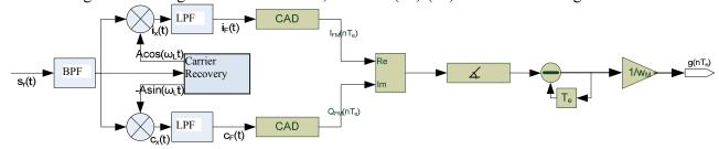
Block diagram of a FM digital demodulator
