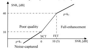
$$\begin{split} P(R(t) < V_0) \approx 1 \Rightarrow \eta = \frac{\rho_0}{\rho_i} = k_3 \cdot 3 \cdot \beta^2 \cdot \frac{BW_{FM}}{2 \cdot f_{mM}}; & \text{for } \rho_i > 10 \Rightarrow \\ SNR_0[dB] = 8.5dB + 10 \lg(3 \cdot \beta^2 \cdot \frac{BW_{FM}}{2 \cdot f_{mM}}) + SNRi[dB] \end{split}$$
