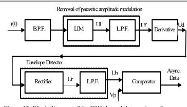
Figure 13. Block diagram of the FSK demodulator using a frequency discriminator
