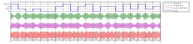
Figure 18. Envelope variations vs. time of QPSK, OQPSK and  $\pi/4$ -QPSK
