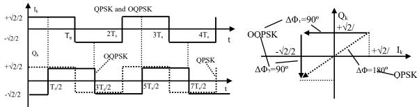
Fig. 14. Relative positioning of the  $I_k$  and  $Q_k$  modulating levels, to generate the QPSK and OQPSK modulations
