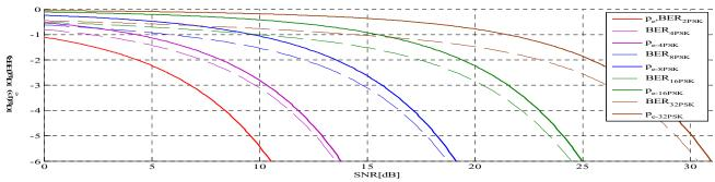
Figure 20.  $p_{e2}$ ,  $p_{e4}$ ,  $p_{e8}$ ,  $p_{e16}$ ,  $p_{e32}$  (continous lines) and BER<sub>2</sub>, BER<sub>4</sub> BER<sub>8</sub>, BER<sub>16</sub>, BER<sub>32</sub>, (daseh lines) vs. SNR Symbol-error probability of the N-PSK
