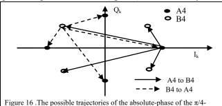
Figure 16 .The possible trajectories of the absolute-phase of the  $\pi/4$ -QPSK starting from a vector of A4 and B4
