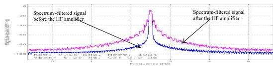
Figure 13 Illustration of the spectral regrowth
