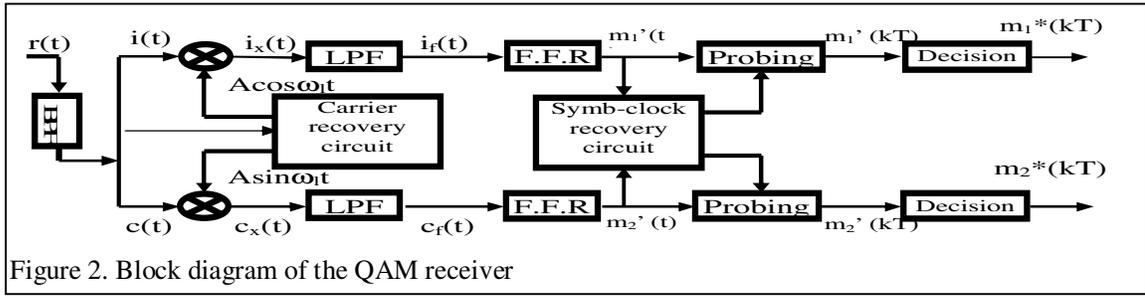
Figure 2. Block diagram of the QAM receiver
