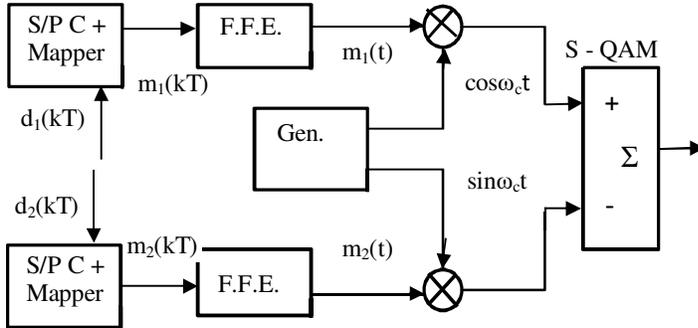
Figure 1. Block diagram of the QAM modulator
