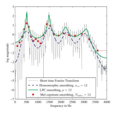
Fig. 5.8 Comparison of spectral smoothing methods.
