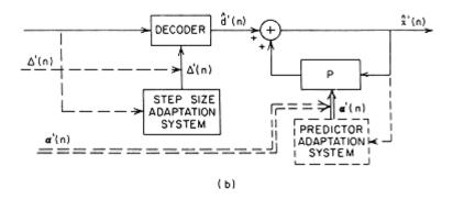
Fig. 7.5 General block diagram for adaptive differential PCM (ADPCM).
