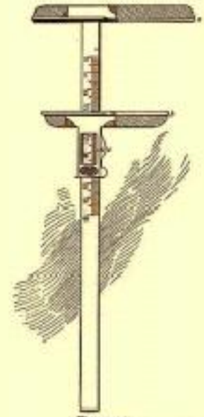
FIGURE 3. SMALL SLIDING COMPASSES.
