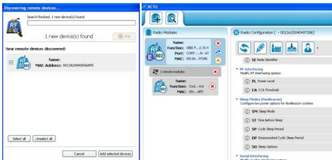
Figure 5. a) Discovering remote devices; b) Read Configuration parameters of the remote device.
