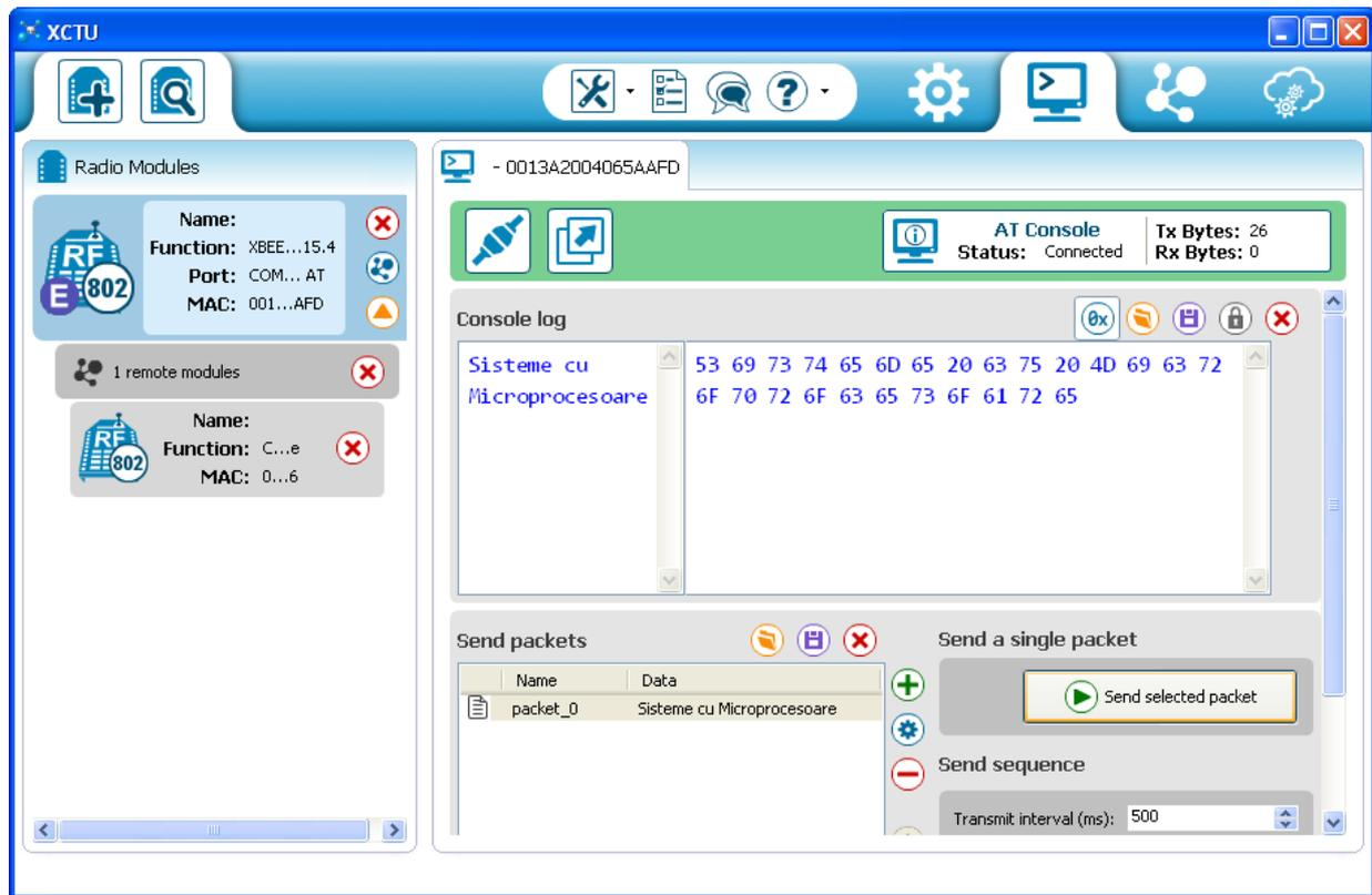
Figure 6. a) Sending packets by remote connection
