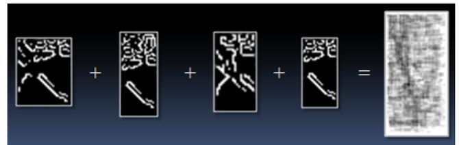
Figure 12. Building a probabilistic model for a pedestrian hand
