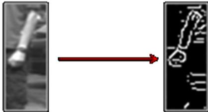
Figure 7. Edge detection of a fragment containing a pedestrian hand
