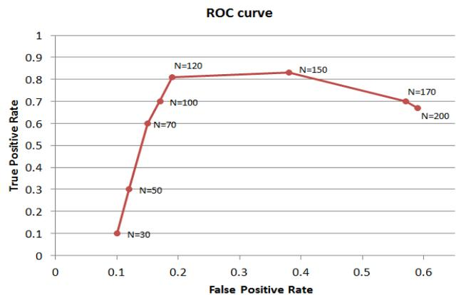
Figure 15. Pedestrian detector ROC curve (performance measurements with different number of fragments  $N$ )
