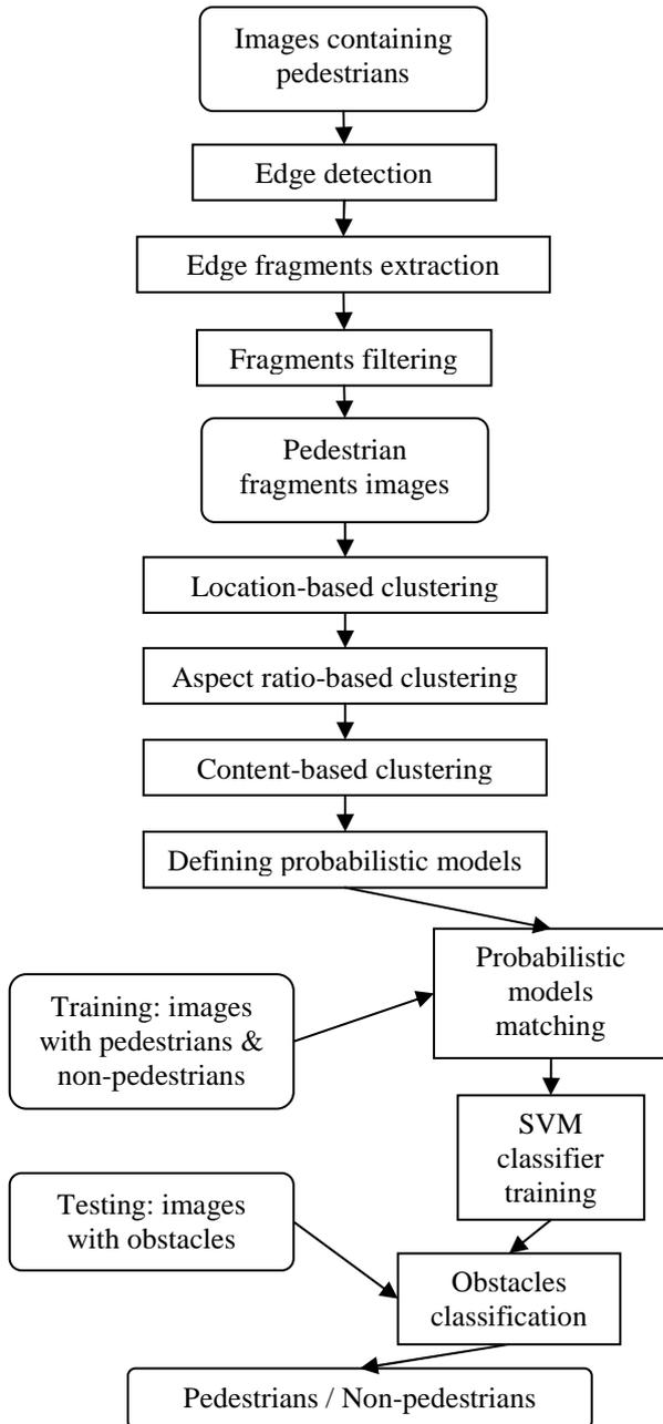
Figure 3. The pedestrian detection system architecture
