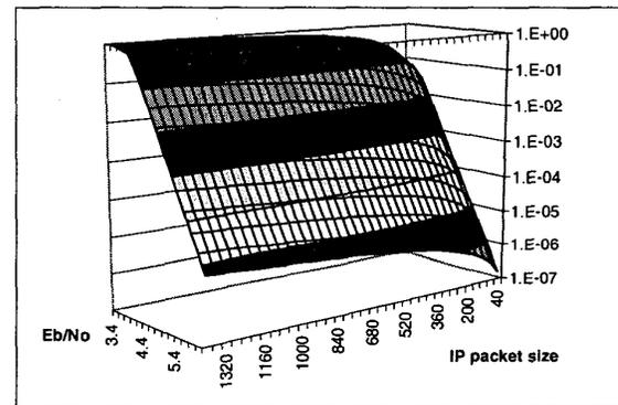
Figure 3C: IP SDU loss ratio in Unacknowledged mode
