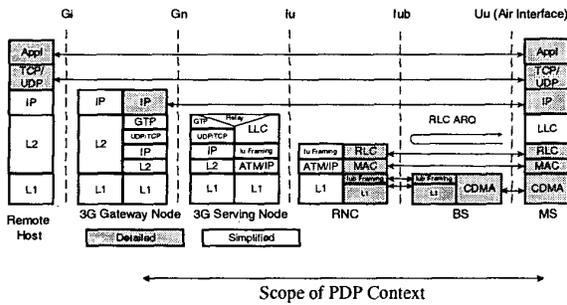
Figure 3A: The user plane protocol stack of the end-to-end scenario of Figure 1A.
