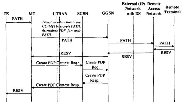
Figure 2A: QoS Signaling Mechanisms in the End-to-end Scenario
