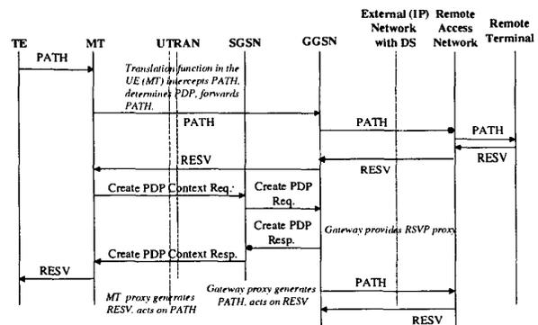
Figure 2B: QoS Signaling Mechanisms in the End-to-end Scenario
