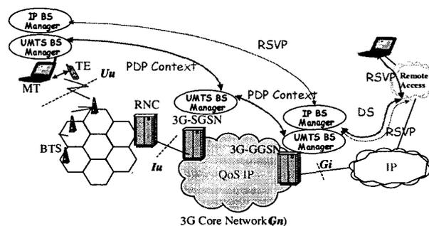
Figure 1A: A 3G End-to-End Scenario with RSVP QoS Signaling
