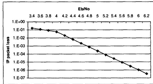
Figure 5A: IP SDU loss ratio in Unacknowledged mode: Fig. 3C "zoomed out" for 80 byte long packets
