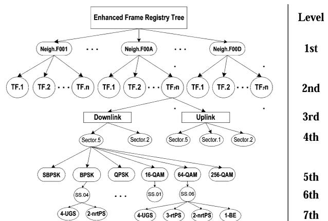
Fig. 2. The enhanced frame registry tree.
