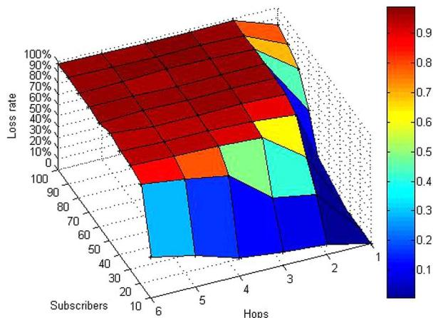
Fig. 11. Multicast video packet loss in the grouped case.
