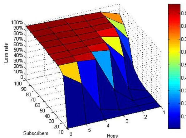
Fig. 10. Unicast video packet loss in the grouped case.
