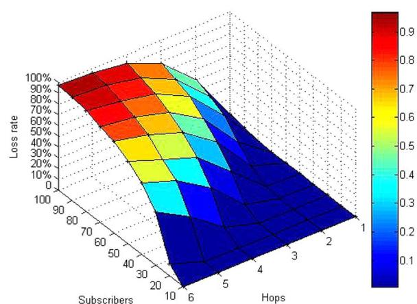
Fig. 12. Voice packet loss in the spread case.
