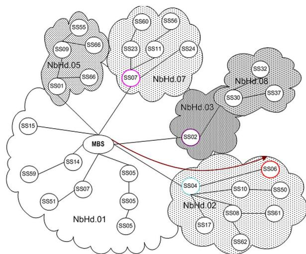
Fig. 1. Example topology of an IEEE 802.16 mesh network.
