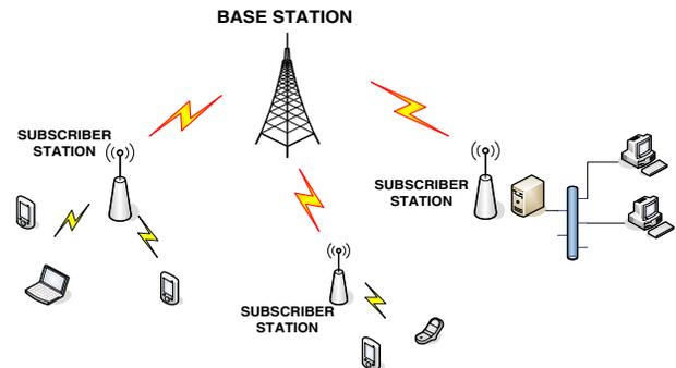
Fig. 1. Example of IEEE 802.16 Wireless Network Topology in PMP Mode.
